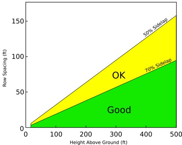
Figure 4: Recommended Row Spacing vs. Height
