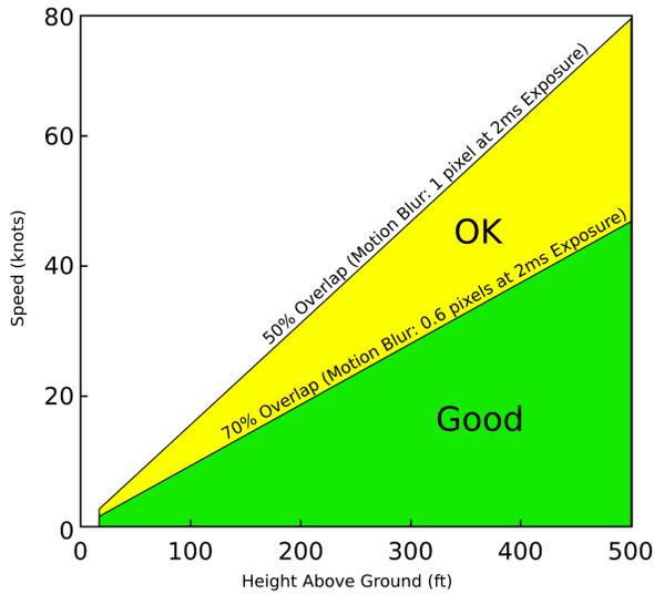
Figure 3: Recommended Flight Profiles
