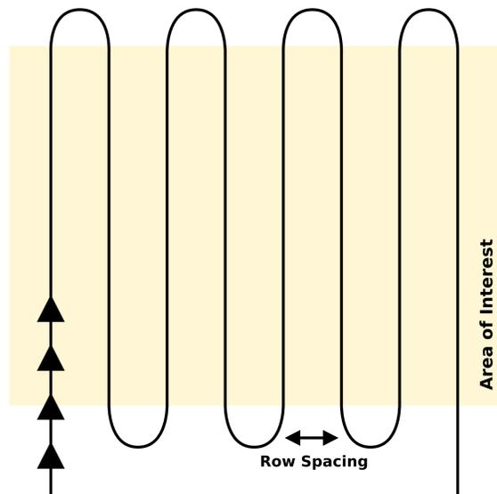
Figure 1: Recommended flight pattern when covering 2D areas.
