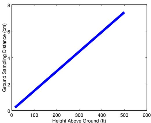
Figure 2: Ground Sampling Distance vs. height
